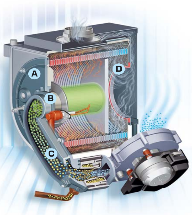
The pre-mixed condensation system of Murelle HE
